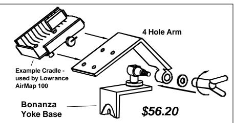
Slips under head of top screw on plate at back of Bonanze yoke (need to remove front plate on Bonanza yoke to restrain holding nut while tightening screw). Use supplied screw and washers if needed to adjust length to avoid interference with other objects inside yoke hub.
