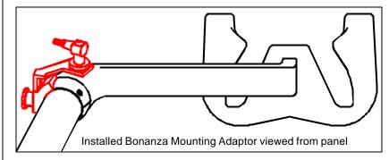
To rotate your Garmin 196\* GPS toward the alternate pilot seat, use the supplied hex key to slightly loosen clamp post screw until post will rotate. Then retighten. Normally rotation back and forth between seats will not loosen threadlocked post screw, but if it does, reset with the hex key.
